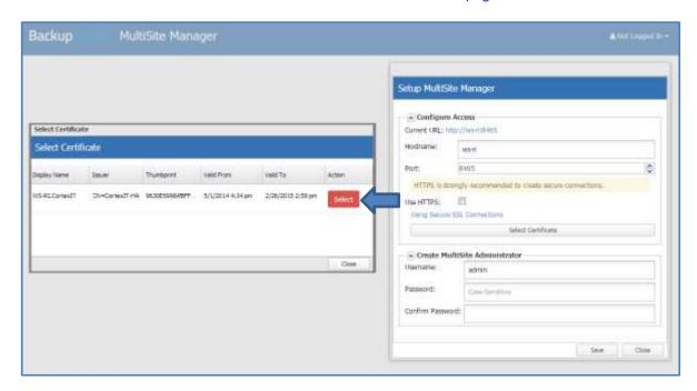
Figure 2: MultiSite Manager setup and SSL certificate selection
