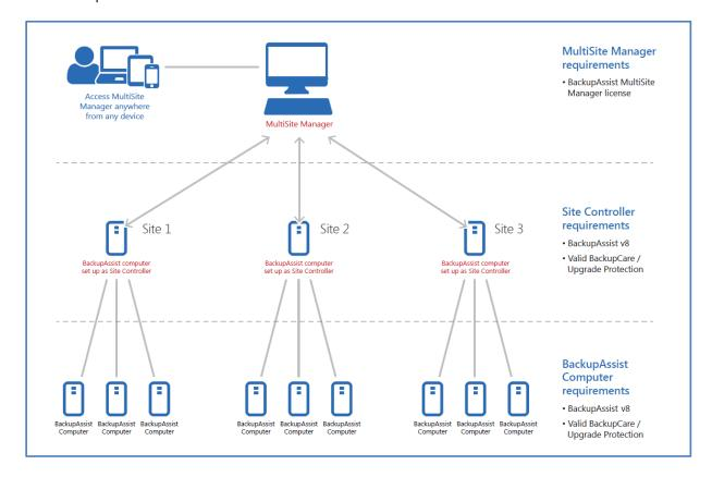
**This diagram** shows the licensing requirements for a MultiSite Manager solution. As you can see, the requirements are clear and consistent for both single-site and multi-site implementations.
